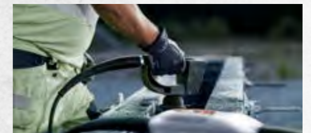
The Smart-E version features a pistol grip handle that reduces hand/arm vibration.
