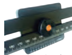
Nonius 1/20 mm reading 1 /20 mm
